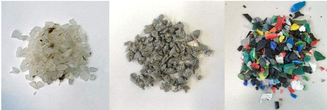
Fig. 1. The tests were carried out on three different materials: pellets of virgin PP (left), PP agglomerate obtained from post-consumer film (center) and regrind obtained from HDPE beverage closures (right).
